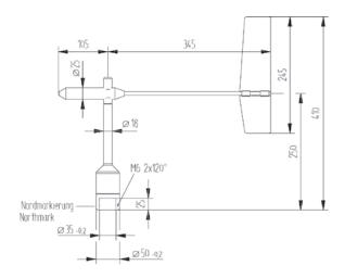
Additionally TMR wind vanes do not have a north gap and thanks to their solid state design they are subject to less mechanical wear that potentiometer wind vanes. TMR wind vanes do not have moving parts, except the bearings.
