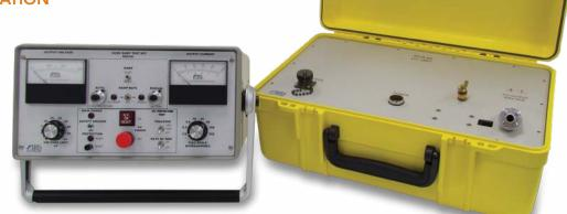
The Iris Power DCR 60-2 is a simple off-line DC tester to identify problems in the stator groundwall insulation system of large AC electric machines before an unexpected in-service failure occurs. Unlike the pass or fail of a DC or AC hi-pot test, the DC ramp test gives diagnostic information and often can be stopped before a failure occurs.
